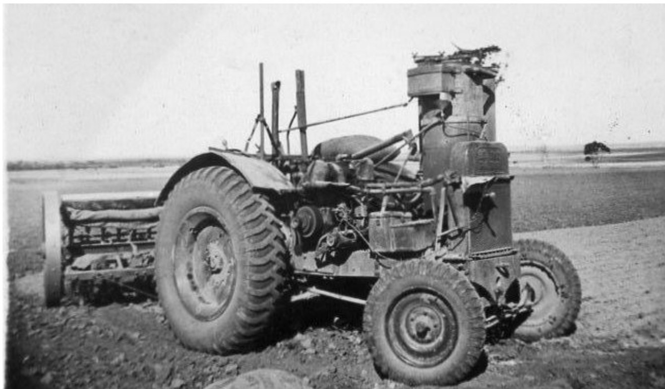
Mr Steve Lundy's Tractor fitted with gas producer
